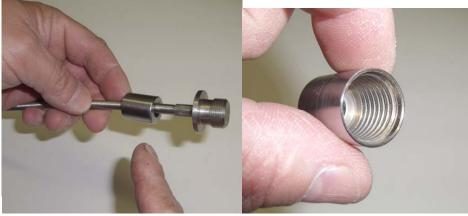
Insert the cable by twisting and pushing and at the same time keep the hose straight.
