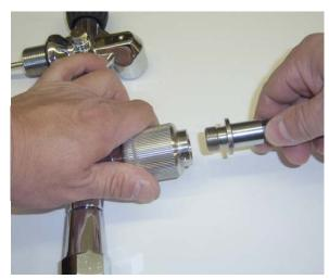
Next remove the knob nut by using an Orifice/Valve T-Handle tool or slotted screw driver.
