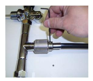
Hold the metal ferrule with a strapping wrench to prevent marring of the metal.
