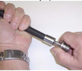
Remove the hose end ferrules. It'll make it easier when you re-insert the cable back in.
