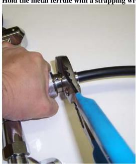
W-D40 can facilitate removal of the knob. Be sure to wash away all of the W-D40 after taking it apart.
