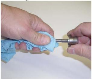
Then, apply silicone grease the full length of the cable.
