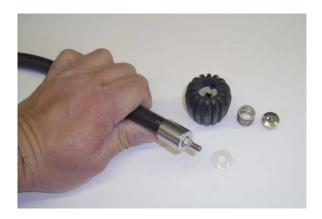
Pull the cable out completely.
