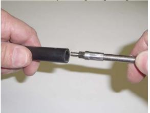
To make it easier to hold, temporarily screw the knob retainer nut on the end, and pull out the last bit of the cable out of the end of the hose.
