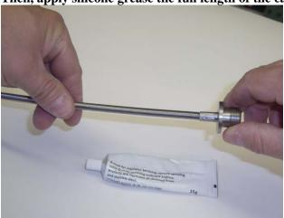
Insert the Hose Ferrule. Notice that they are threaded. So, thread it all the way; flush to the hose.
