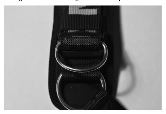
Step 4 Install a Triglide and D ring above the 1 inch sewn webbing
